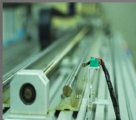
Limit Switch Sensor
